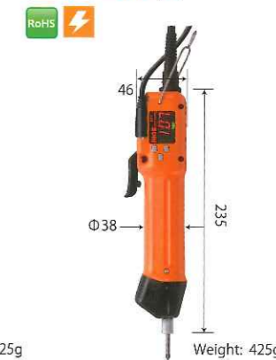
Lever and Push-to start (two-way) BLG-5000BC2-20 (Rotation Speed: 2.000r.p.m)
